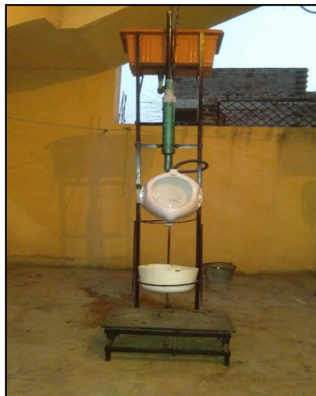
Fig 1.1: Fabricated model of Automatic Flushing System
